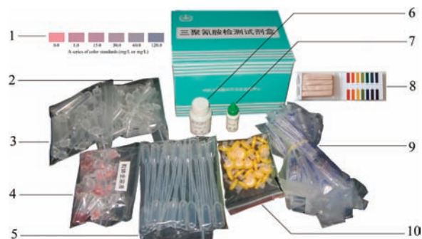
Figure 1. Composition of the rapid detection kit for Mel. The kit is composed of the following reagents and materials: (1) standard colorimetric card; (2) microtube (2 mL); (3) microtube (5 mL); (4) Au NP solution (300 \mu\text{L}/\text{tube} ); (5) plastic straw (1 mL); (6) trichloroacetic acid (300 g/L); (7) NaOH (3 M); (8) pH testing strip; (9) syringe (1 mL); (10) filter.
